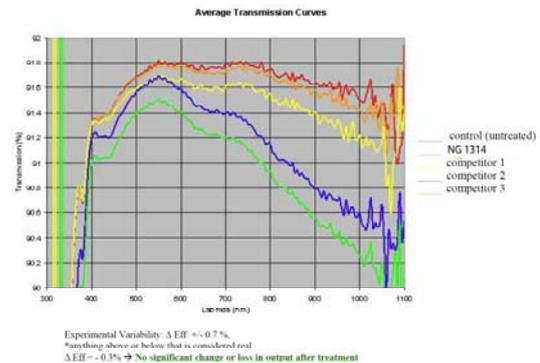
**NG 1314/D** has undergone independent testing with solar panel manufactures to ensure light transmission through the treated glass is not affected. The coating is invisible, treated glass is almost as transparent to the spectrum of the light than completely untreated glass.
