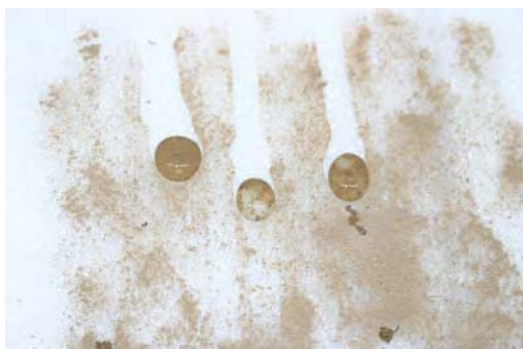
Water droplets pick up dust and dirt from a treated test panel. (self cleaning effect)
